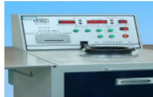
Air Permeability Test
